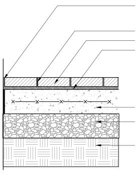
EXPANSION JOINT AT STRUCTURES, CURBS, WALLS. KEEP TOP OF JOINT FILLER BELOW PAVERS. CAULK AND SEAL AS NEEDED. MORTAR OR SAND JOINTS BRICK OR GRANITE PAVERS 3/4" SAND/ CEMENT (3:1) SETTING BED
