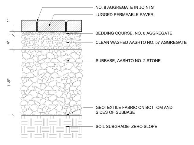
PERMEABLE PAVEMENT SYSTEM: SECTION
