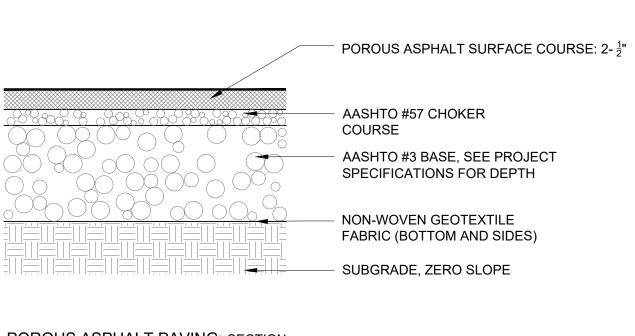
POROUS ASPHALT PAVING: SECTION
