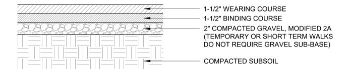
ASPHALT PAVING: SECTION
